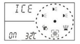
Freezing water temperatures can cause damage to equipment in the spa. The spa includes a winter mode to prevent this. When water temperature drop below 5°C the heater will turn itself on to raise the temperature of the water to 8°C.
