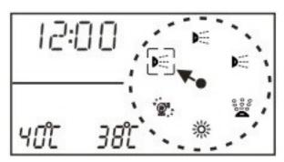
To turn on a feature in the Hot Tub, simply press the to move the arrow, then press OK to turn your selected feature on or off.
